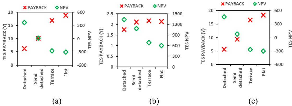
Figure 8. Payback and NPV associated with TES investment for (a) non-incentivised design, (b) incentivised design (FIT), and (c) incentivised design (CO<sub>2</sub> levy exemption)
