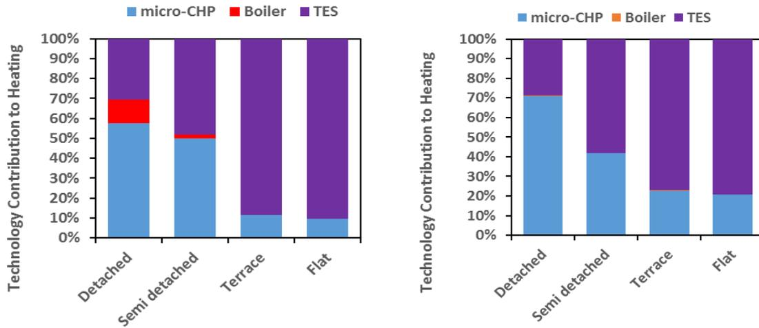
Figure 4. Non-incentivised design with TES Figure 5. Incentivised design (FIT) with TES
