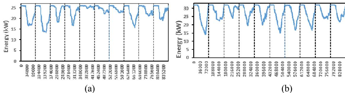
Figure 6. TES discharge profile for non-incentivised design (a) detached house, (b) flat
