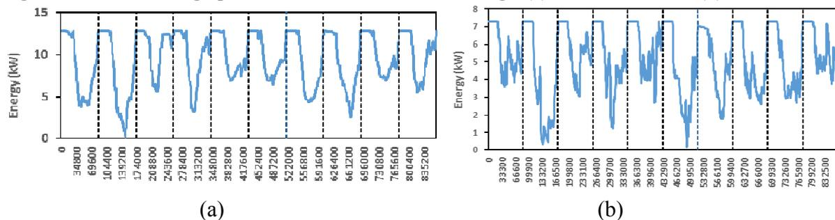
Figure 7. TES discharge profile for incentivised design (a) detached house, (b) flat
